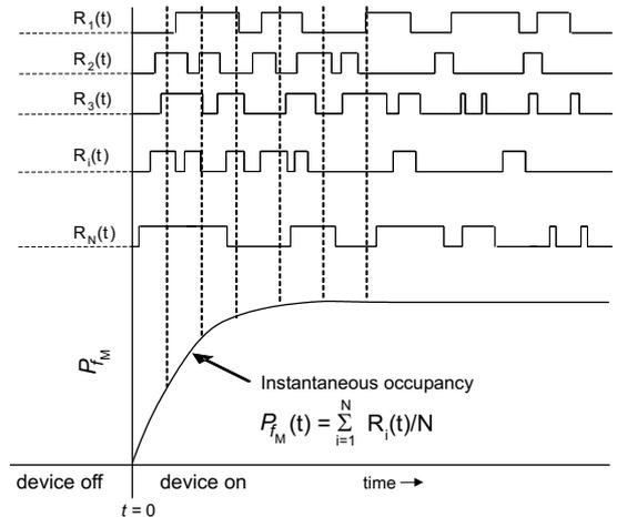
Fig. 3. Schematic representation of the instantaneous measured occupancy  $P_{fM}(t)$ .
