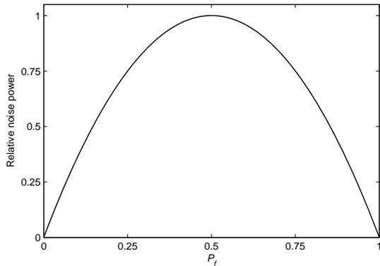
Fig. 2. Relation of trap-occupancy with RTS noise power.
