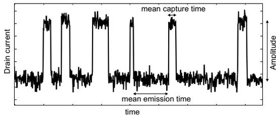
Fig. 1. Time domain sample of the drain current of a MOSFET ( $W/L = 1/0.13\mu\text{m}$ ).
