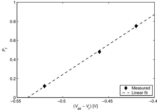
Fig. 8. Measured OFF-state occupancy at different gate OFF-voltages, after a constant OFF-time ( $t_{\text{off}} = 5$  ms).
