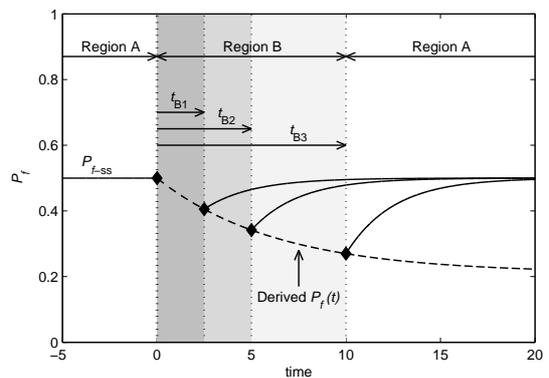
Fig. 6. Extraction method for the occupancy of regime B.
