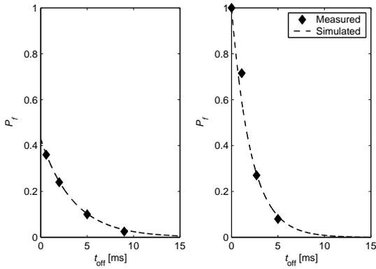
Fig. 7. Measured and simulated OFF-state occupancy. Extracted time constants: a)  $\bar{\tau}_e = 3.5$  ms,  $\bar{\tau}_c \gg \bar{\tau}_e$ . b)  $\bar{\tau}_e = 2.0$  ms,  $\bar{\tau}_c \gg \bar{\tau}_e$ .
