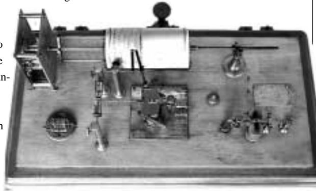
Lightning recorder: "The trembler not only rang the bell and vibrated the coherer, but also deflected the recorder pen."
