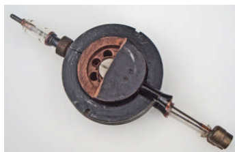
Cut-open experimental Cavity Magnetron designed by GEC for World War 2 radar photo © Tony Dutton
