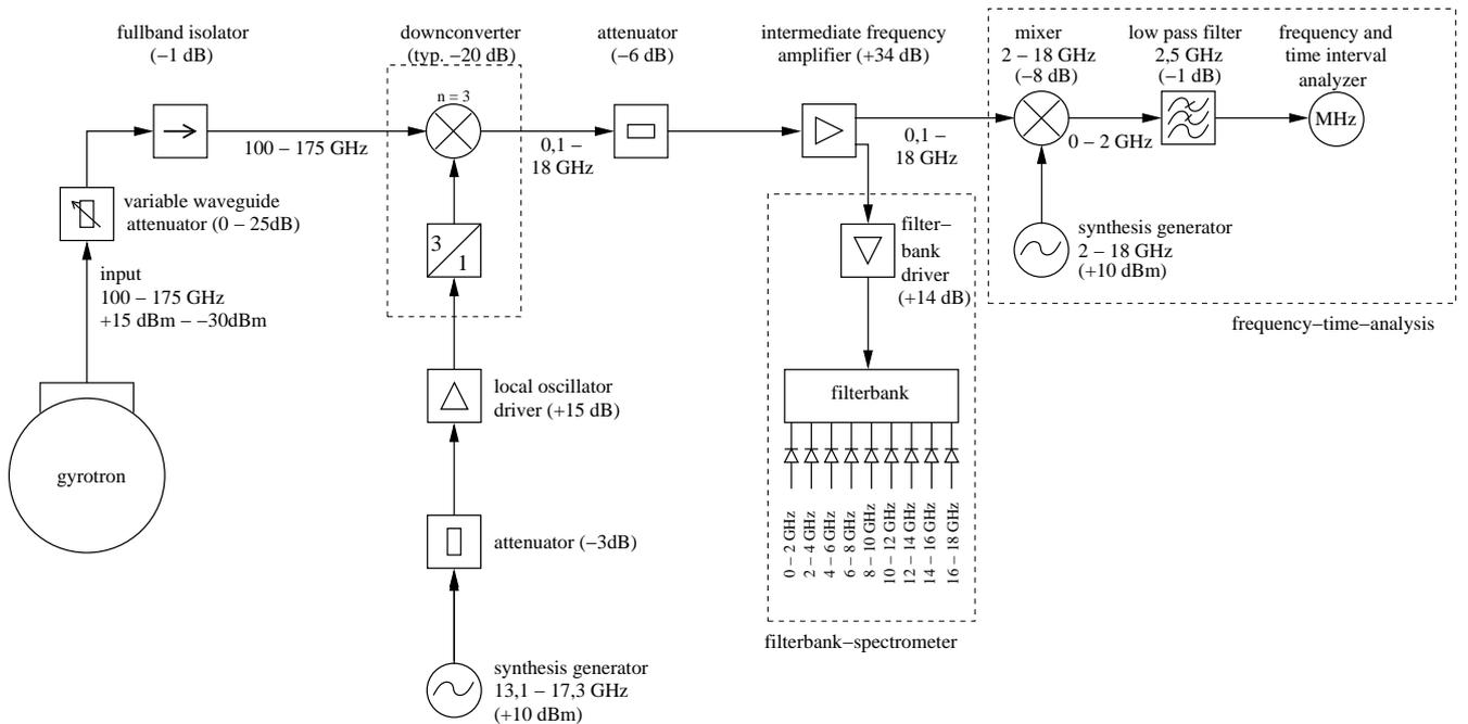
Fig. 2. Block diagram of the frequency measurement system with filterbank spectrometer and frequency time analysis.
