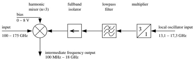
Fig. 3. Block diagram of the downconverter.
