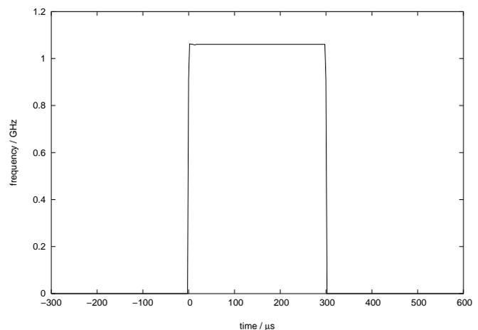
Fig. 5. Gyrotron frequency measured on the IF by the frequency and time interval analyzer.
