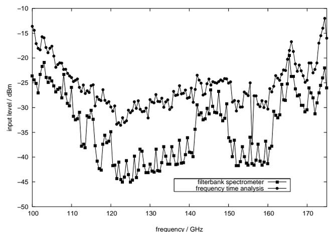
Fig. 6. Sensitivity of the filterbank spectrometer and the frequency time analysis.
