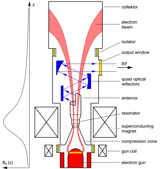
Fig. 1. Cross section of a gyrotron with radial output.
