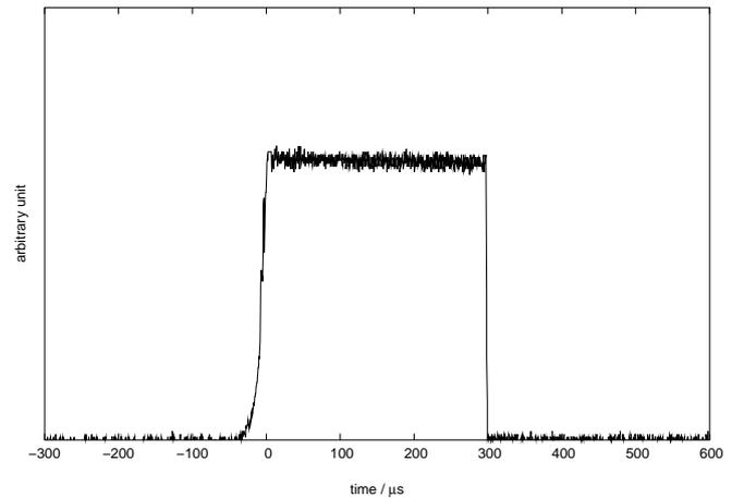
Fig. 4. Output of the filterbank spectrometer; IF: 8 GHz – 10 GHz, RF: 138.95 GHz – 140.95 GHz.
