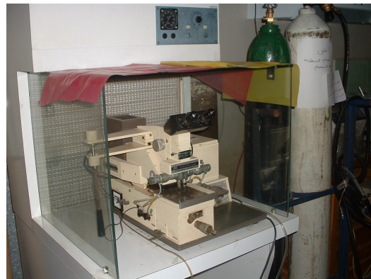
Fig.3. The mask aligner used for the sample exposure to UV radiation.
