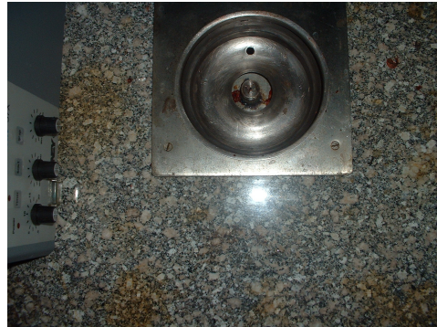
Fig.2. The spin coater used during the photoresist application to obtain a uniformly deposited photoresist layer.
