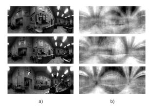
Fig. 2. a) A sample of images from the sequence taken with the mobile robot in a laboratory. The images have been transformed into the cylindrical form. b) First three principle components (eigenvectors).
