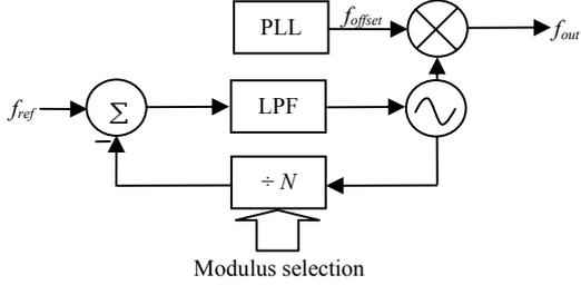
Fig. 5. Block diagram of a dual (parallel connected) loop topology with the SSB mixer placed on the output of the two synthesizers.
