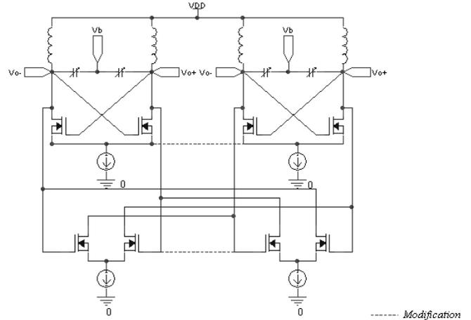
Fig. 16. Coupled LC oscillators with quadrature outputs
