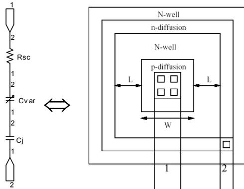
Fig. 15. Basic model and layout of the varactor.
