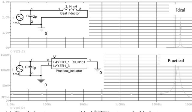
Fig. 14. Simulation to compare an ideal inductor to a spiral inductor.
