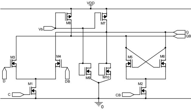
Fig. 10. A full-speed SCL latch.
