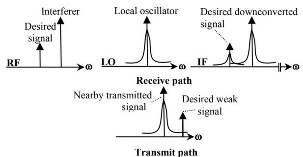
Fig. 1. Effect of phase noise on receive and transmit paths.
