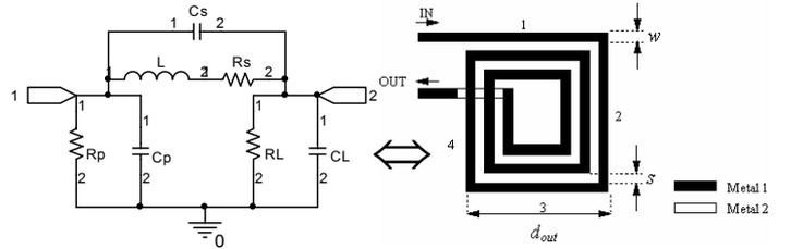
Fig. 13. Simplified model and layout of the inductor.
