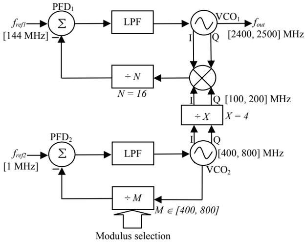
Fig. 6. Concept design and frequency planning of the synthesizer.
