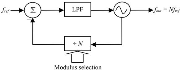
Fig. 2. Block diagram of a single loop integer- $N$  topology.
