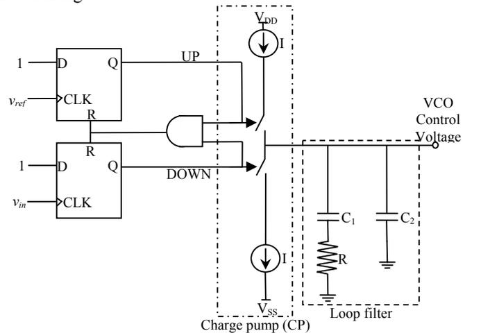
Fig. 8. A PFD with a charge pump output stage.
