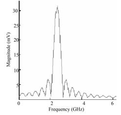
Fig. 7. Spectrum obtained from simulation of the mathematical (SIMULINK) model.
