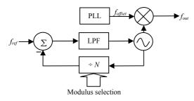
Fig. 5. Block diagram of a dual (parallel connected) loop topology with the SSB mixer placed on the output of the two synthesizers.
