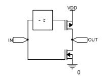
Fig. 19. Conceptual diagram of the negative delay skew idea.
