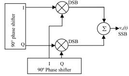
Fig. 12. Block diagram of the SSB mixer.
