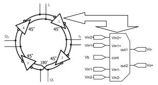
Fig. 18. Block diagram of a conventional four-stage ring oscillator.
