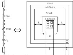
Fig. 15. Basic model and layout of the varactor.
