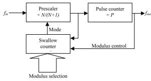
Fig. 11. Block diagram of the programmable divider.
