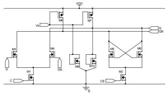
Fig. 10. A full-speed SCL latch.
