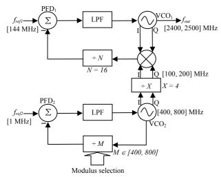
Fig. 6. Concept design and frequency planning of the synthesizer.
