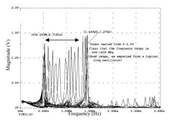
Fig. 20. Simulation result obtained by doing a dc voltage (VCO control) parametric sweep on the ring oscillator circuit.
