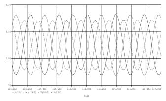
Fig. 17. Time domain simulation result from the LC oscillator circuit.
