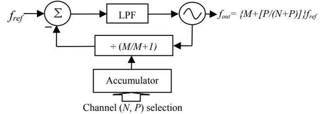
Fig. 3. Block diagram of a fractional- $N$  topology.
