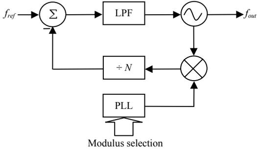
Fig. 4. Block diagram of a dual (series connected) loop topology with the SSB mixer placed within the upper-loop.
