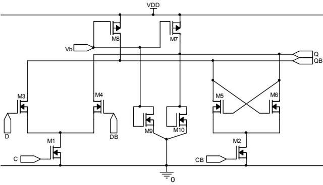
Fig. 10. A full-speed SCL latch.
