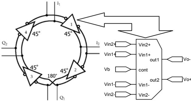
Fig. 18. Block diagram of a conventional four-stage ring oscillator.
