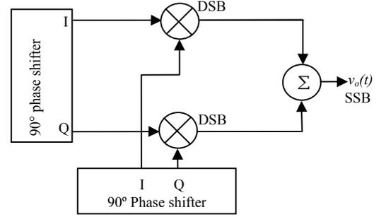
Fig. 12. Block diagram of the SSB mixer.
