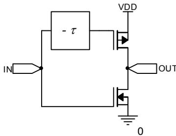
Fig. 19. Conceptual diagram of the negative delay skew idea.
