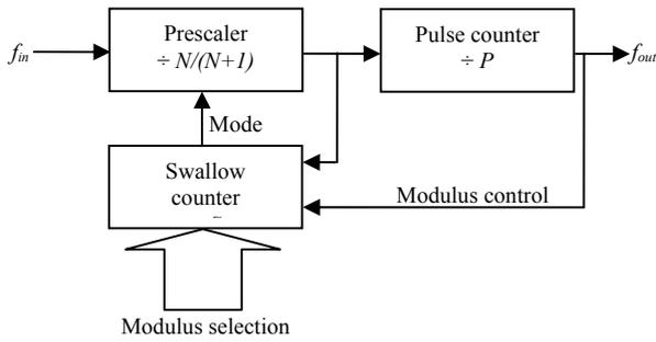
Fig. 11. Block diagram of the programmable divider.
