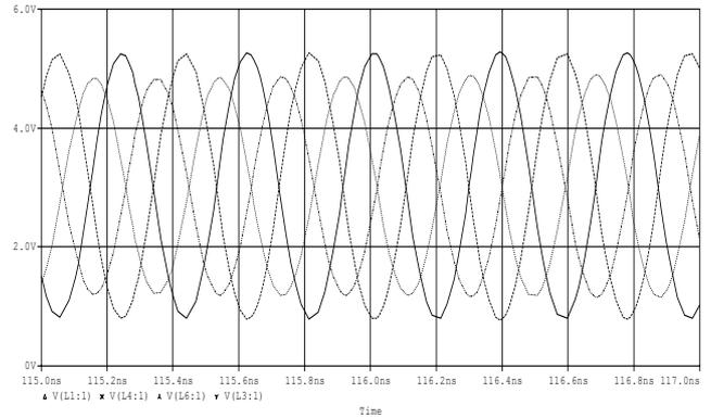
Fig. 17. Time domain simulation result from the LC oscillator circuit.
