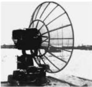
Transmit antenna of Zenit L-band 3D pulsed radar (1938-1943)
