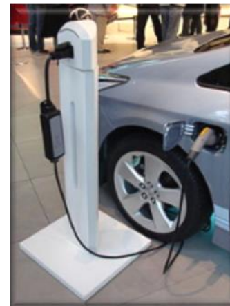
e.g. 2030.1.1: DC quick charger for EV
